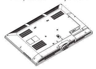
**2** Secure the stand to the screen with the four provided screws.
